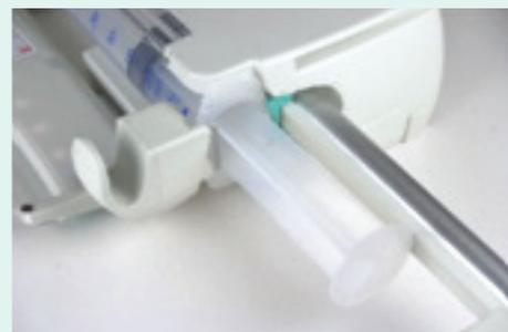
4. Return Syringe Holder to closed position and close the pump door (fig B).
