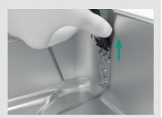
I Condensate outlet undamaged. Gaskets (housing and bellows) intact.
