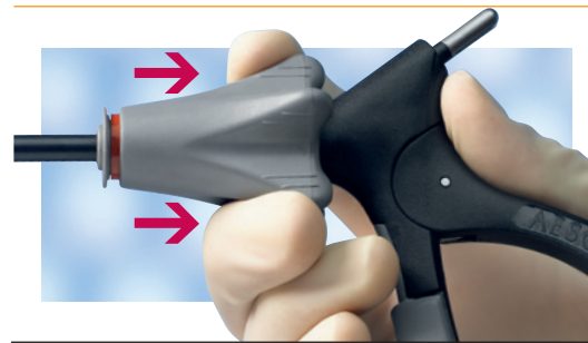
II Disconnect shaft and handle Pull rotation knob back until it locks in place. A red ring becomes visible. Important: Do not hold on to the movable handle component.
