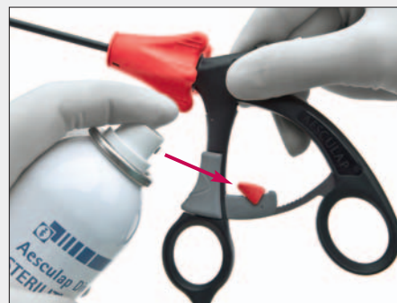
Lubricate the parts of the instrument specified (jaws and red toggle switch) with Aesculap Sterilit Oil after each cleaning cycle.
