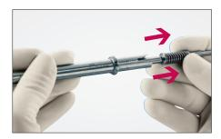
5. Pull inner tube out of outer shaft.
