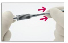
6. Pull push rod out of inner tube.
