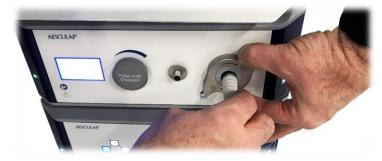
Rotate cable release clockwise and pull light lead, to remove from light source
