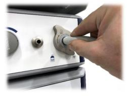
Rotate clockwise to increase light output
