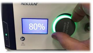
Press light source control to activate / Deactivate light output
